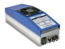
Mount the charger on a flat surface as shown on the image. The device can withstand higher stress due to vibration and shock in the horizontal position.
